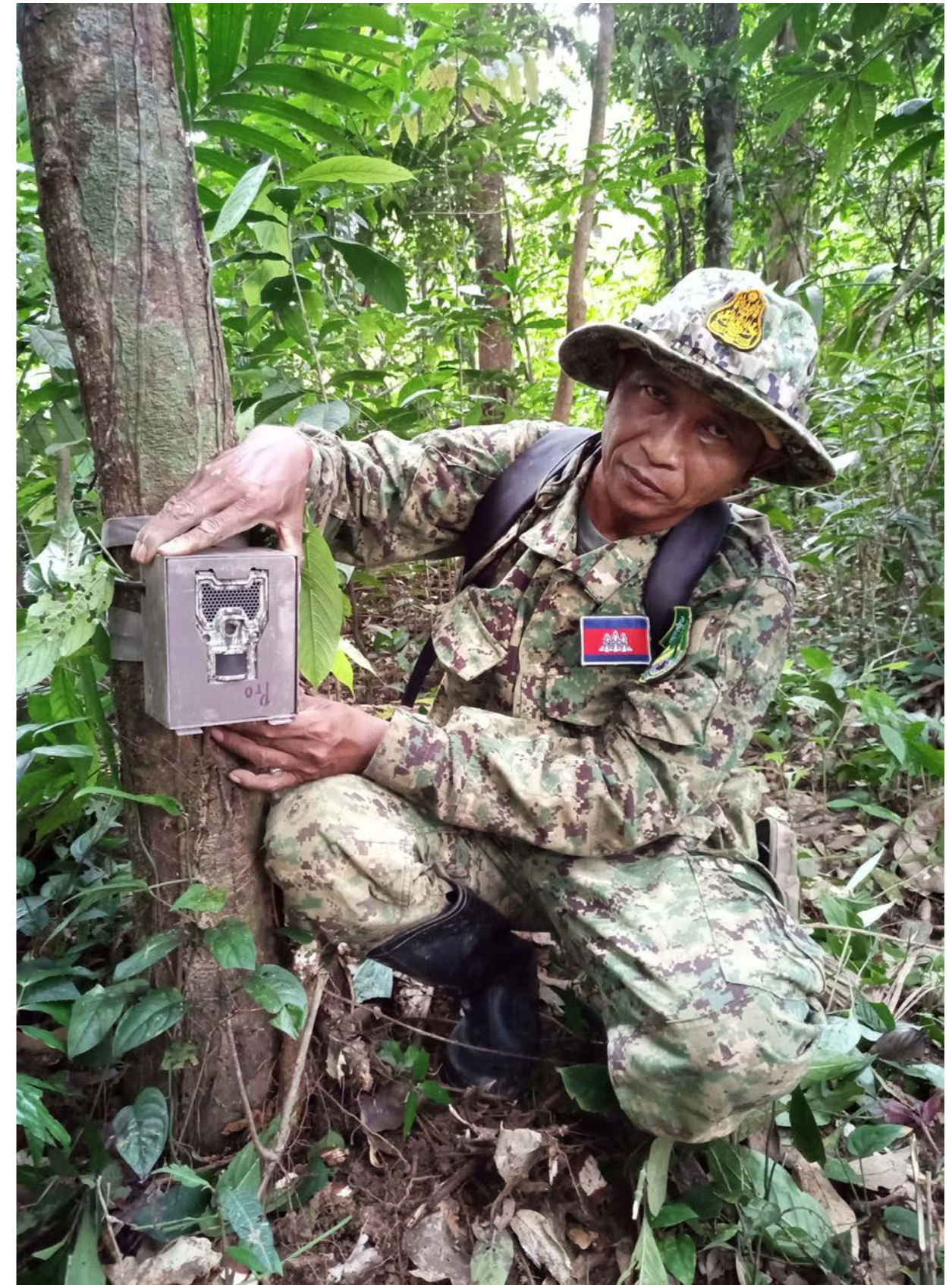
Fig. 2: Installation of camera trap in its protective metal box
