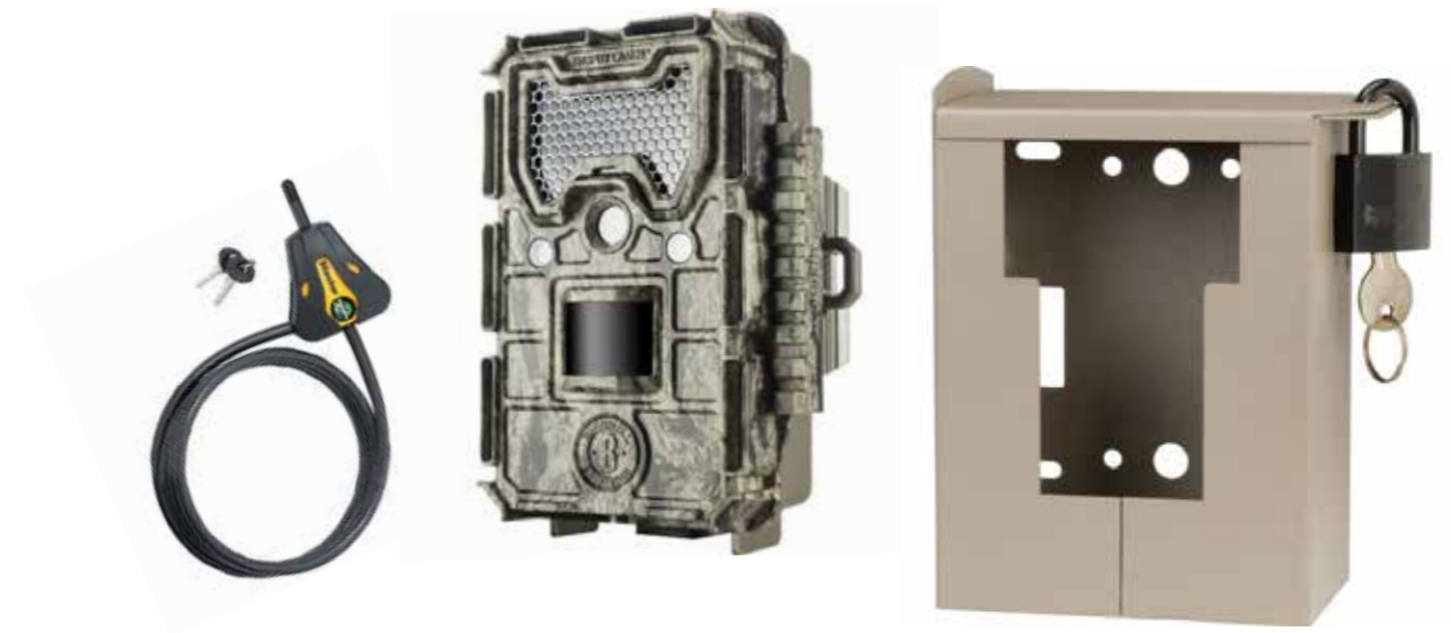
Fig. 1: The survey used Bushnell 24MP Trophy Cam HDs units with python lock and protective housing.
